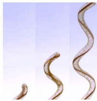
Figure 2.201- Vine robot elongating twice as much as its original length (reprinted with permission from vinerobots.org)
